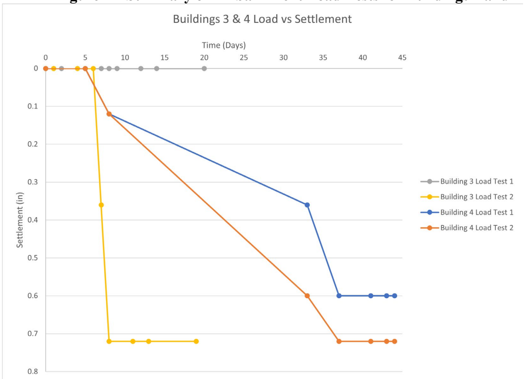
Figure 5 – Summary of Embankment Load Tests for Buildings 3 and 4
