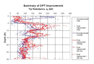
Figure 6 – CPT Tip Resistance Comparison
