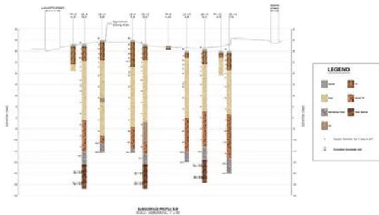
Figure 3 – Generalized Soil Profile
