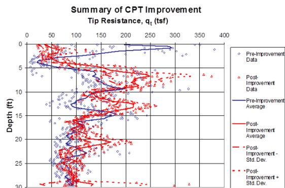
Figure 6 – CPT Tip Resistance Comparison
